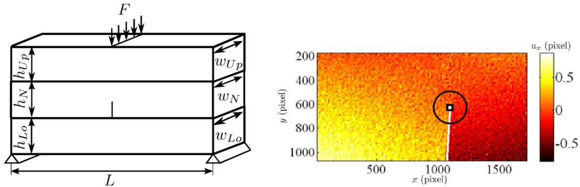
Figure 1. Sandwich-Beam test in which the rock sample is loaded with two aluminum alloy beams (left). Measured horizontal displacement field (expressed in pixels) when rigid body translations have been removed (right), after Guy et al. (2018)
