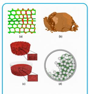
a) BBP modeling of tensile fracture of plant tissue [8] - WP1. b) Simulation of particle fracture [11] - WP2. c) and d) Modeling of fragmentation under axial compression [12] and Fragmentation of grains in a ball mill (particle damage is shown from light to dark green) [13] - WP3.
