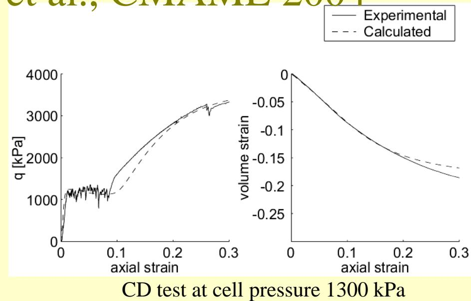
CD test at cell pressure 1300 kPa
