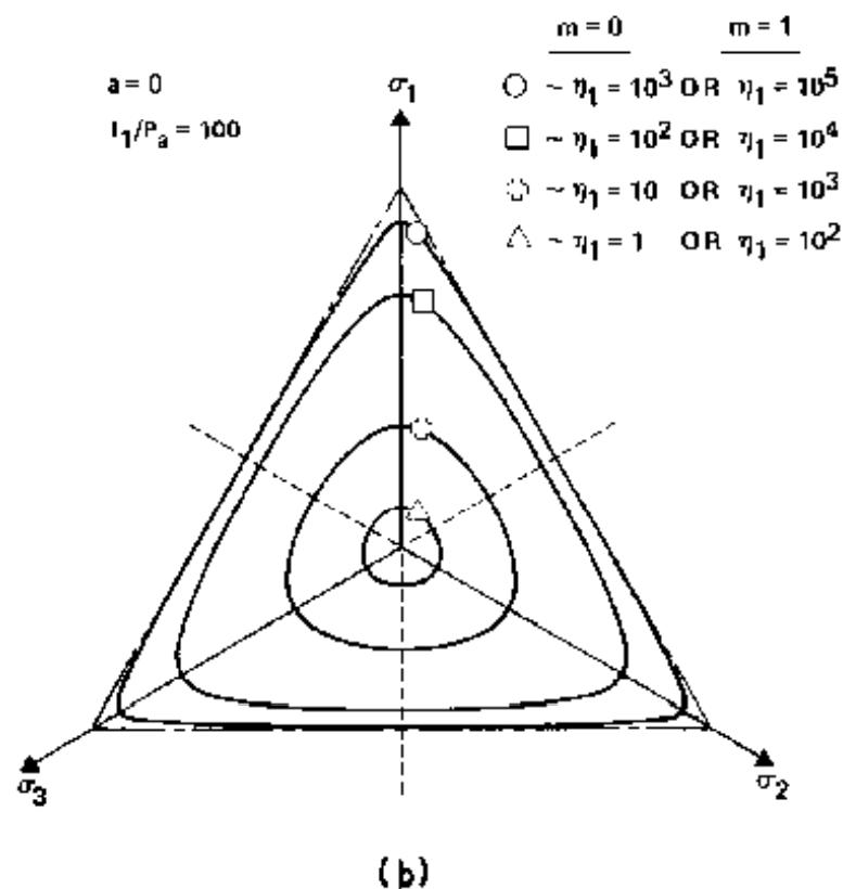
Figure 5. Characteristics of failure surfaces shown in principal stress space. Traces of failure surfaces shown in (a) triaxial plane and in (b) octahedral plane
