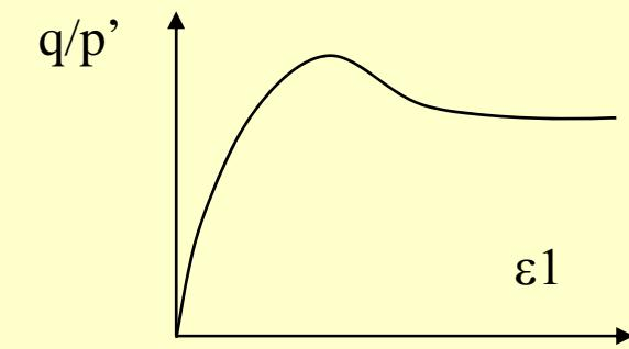
Liquefaction (very loose sand, undrained)
