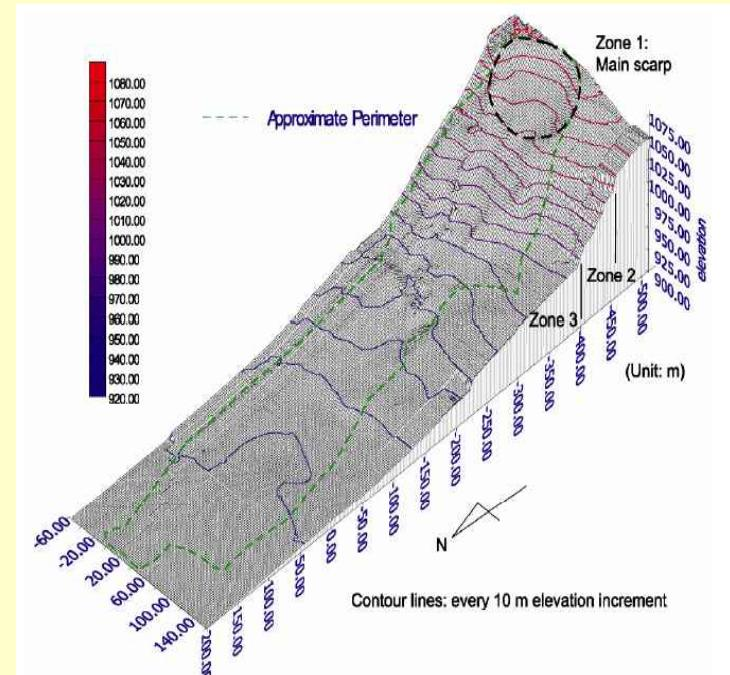
Figure 2.13 Surveyed Slope plotted with surfer with green dashed perimeter.
