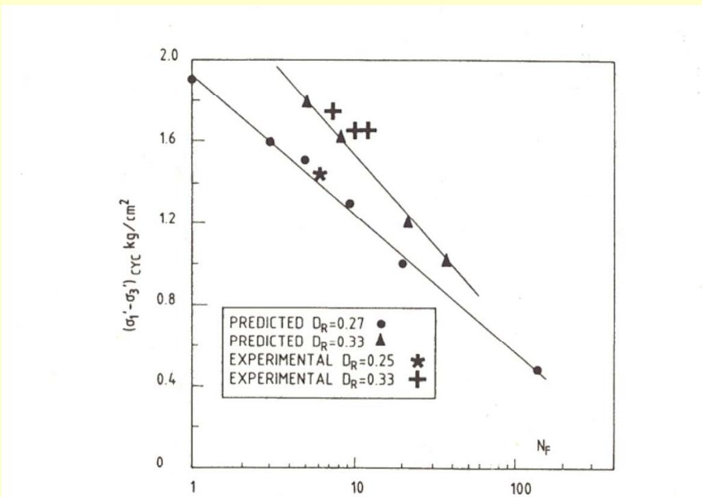
Figure 15. Influence of cyclic deviatoric stress on the number of cycles to cause liquefaction
