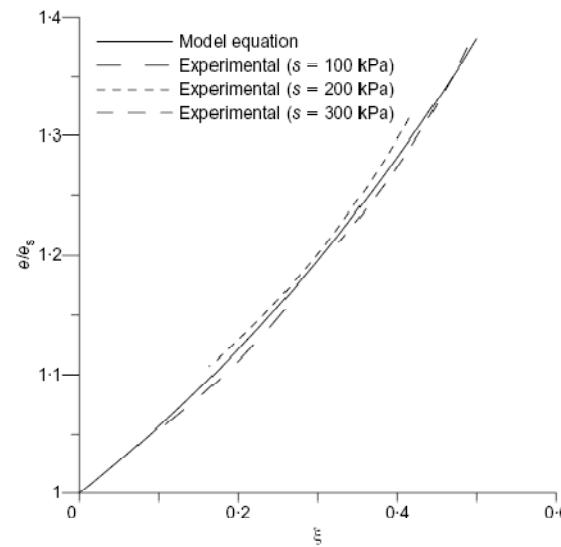
Isotropic compression lines at constant suction (left) and
