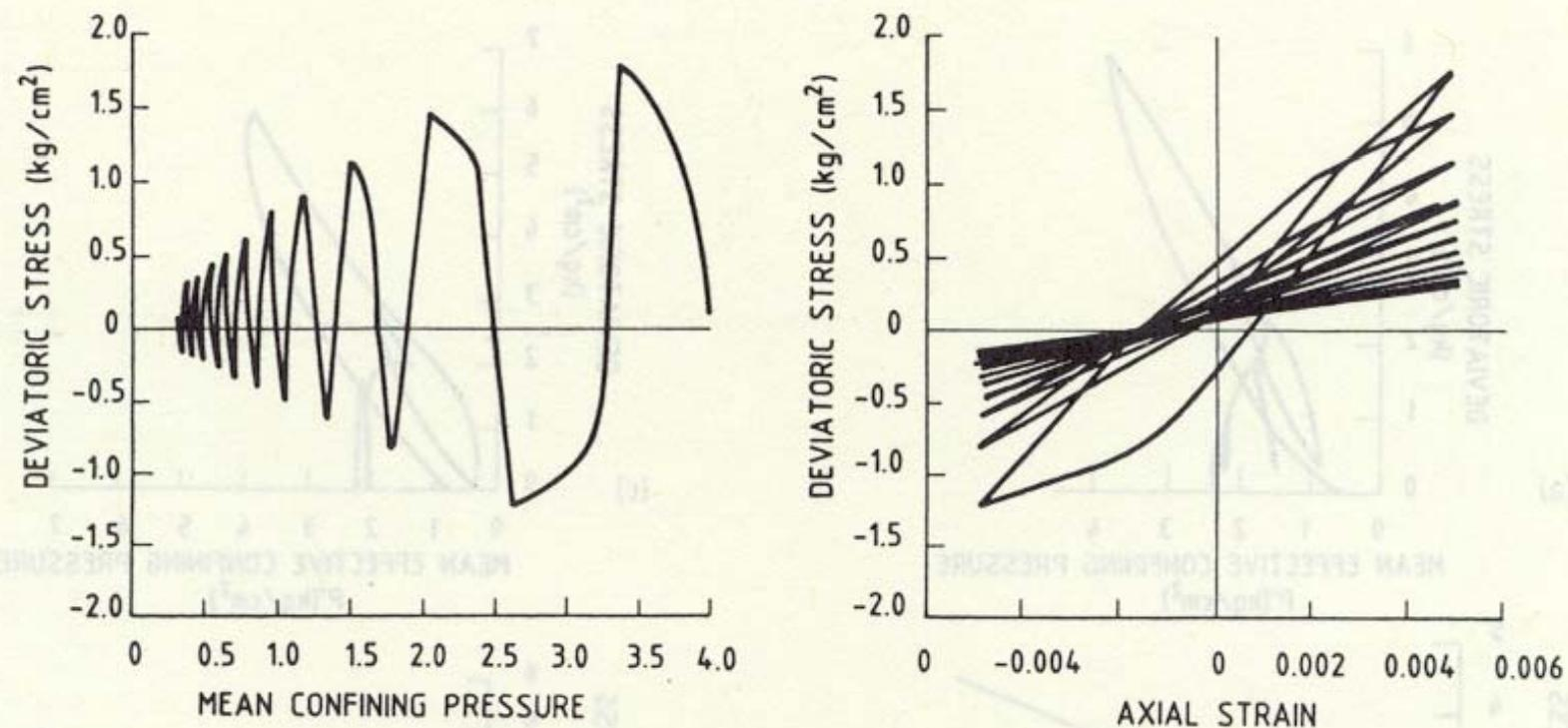
Figure 14. Strain-controlled cyclic triaxial test on loose Banding sand (predicted)
