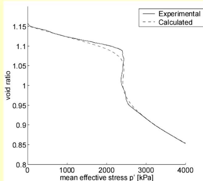
Isotropic compression test
