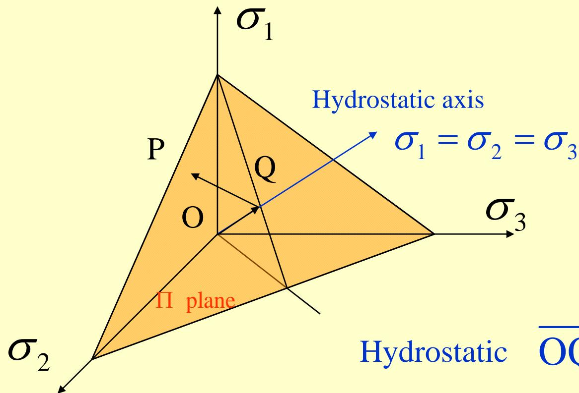
Hydrostatic  $\overline{OQ} = \frac{I_1}{\sqrt{3}} = \sqrt{3}p$
