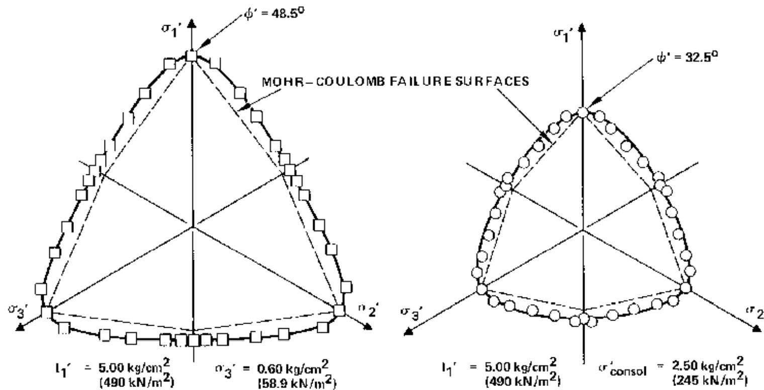
Figure 9. Comparison of failure criterion with experimental results of cubical triaxial tests projected on common octahedral planes for (a) dense Monterey No. 0 sand by Lade,<sup>10</sup> and for (b) normally consolidated, remolded Edgar plastic kaolinite by Lade and Musante<sup>18</sup>
