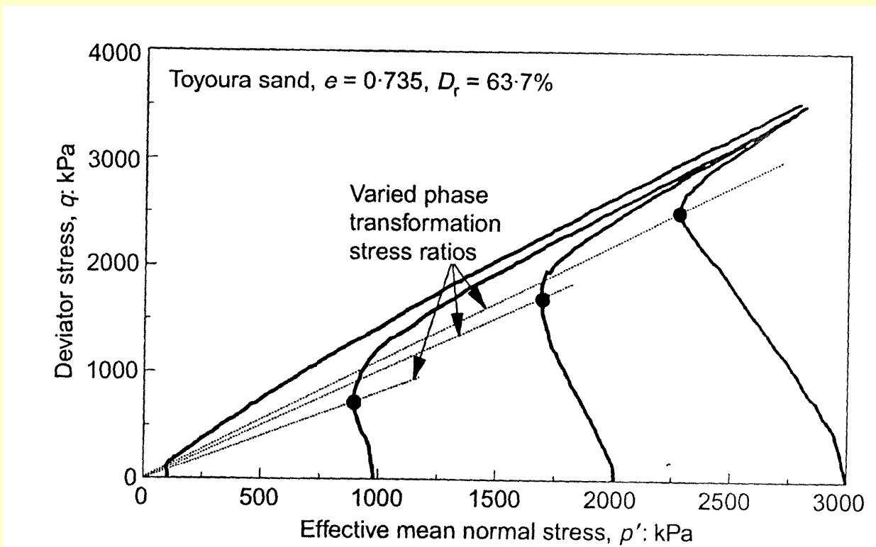
**Fig. 5.** Variation in the phase transformation stress ratio with material state (data from Verdugo & Ishihara (1996))
