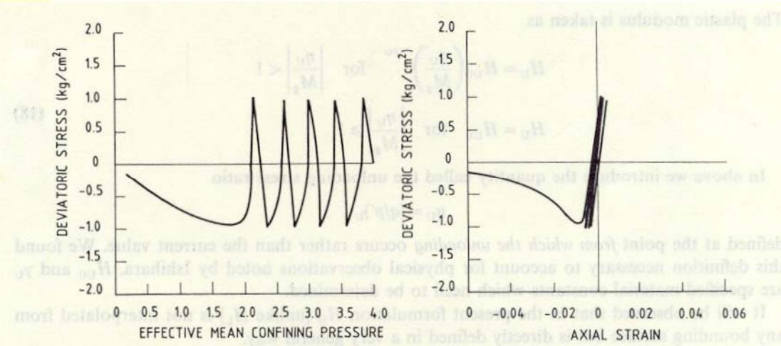
Figure 13. Liquefaction of Banding sand under two-way cyclic loading (predicted)
