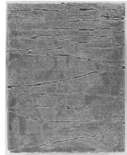
Spalling failure in Berea sandstone specimens. The dimensions of the specimen are height 90 mm and length 110 mm
