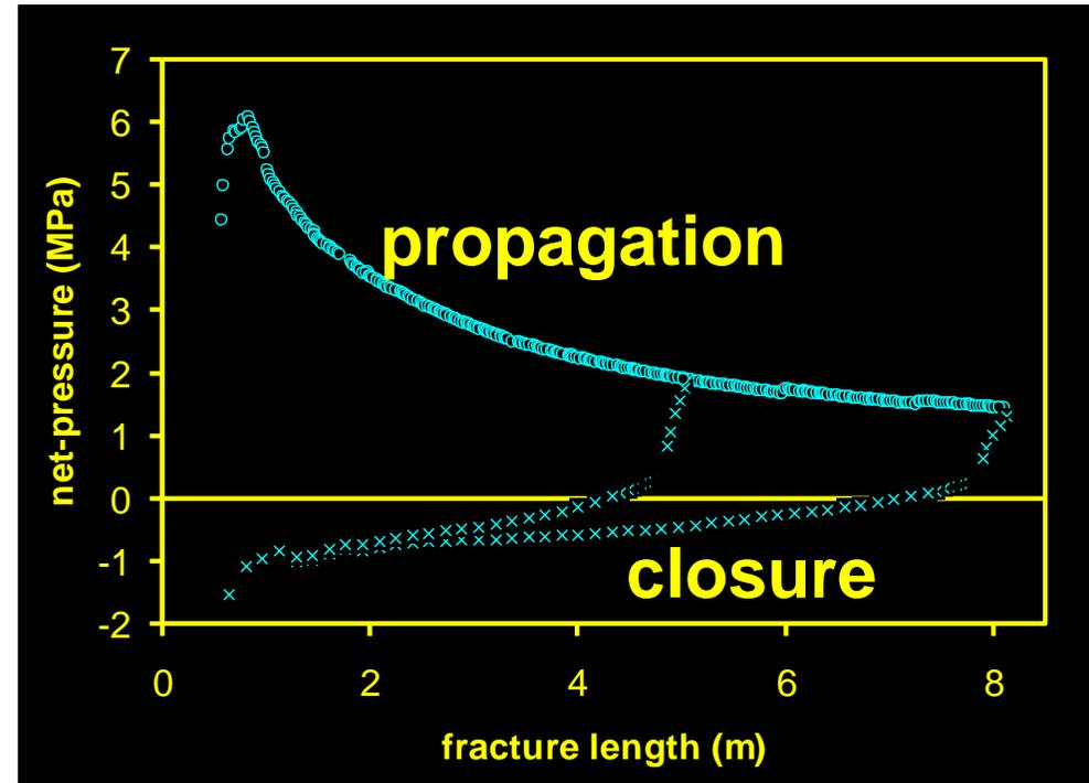
Plastic fracture closes first near the tip
