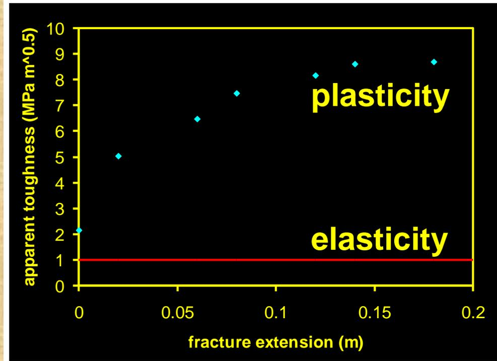
Propagating pressures are higher in plastic fractures
