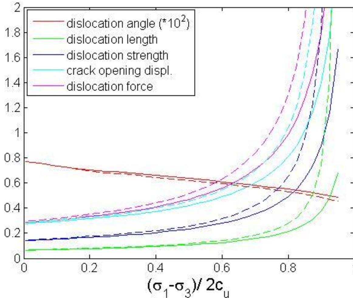
Dimensionless quantities vs ductility number for an undrained material for small scale yielding (solid lines) and large scale yielding (dashed lines).
