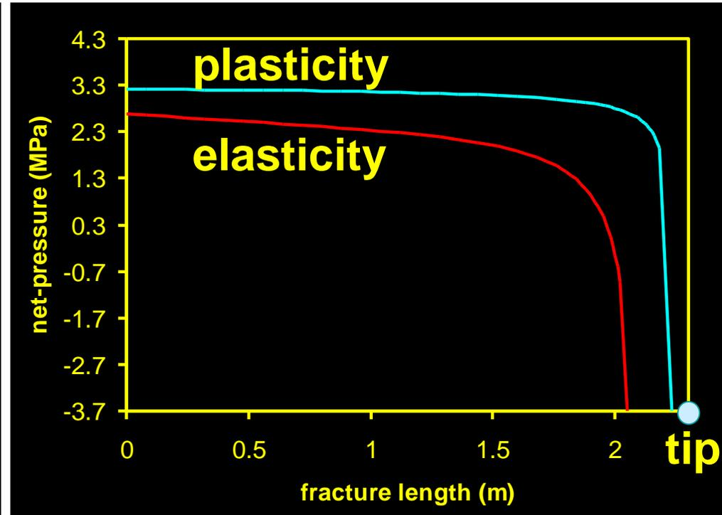
Plastic fractures are wider and shorter than the elastic fractures
