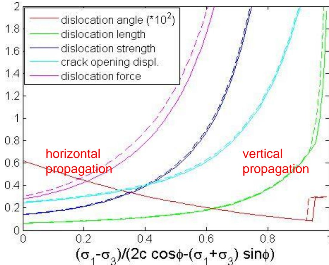
The values between 0 and 1 correspond to fracture propagation of increasing ductility from brittle to small and large scale yielding and finally to 1 for a fracture that requires infinite energy release per unit advance
