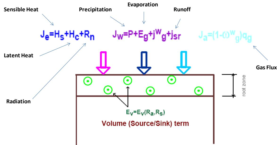
Mass balance of heat (including conductive, diffusive and advective fluxes)
