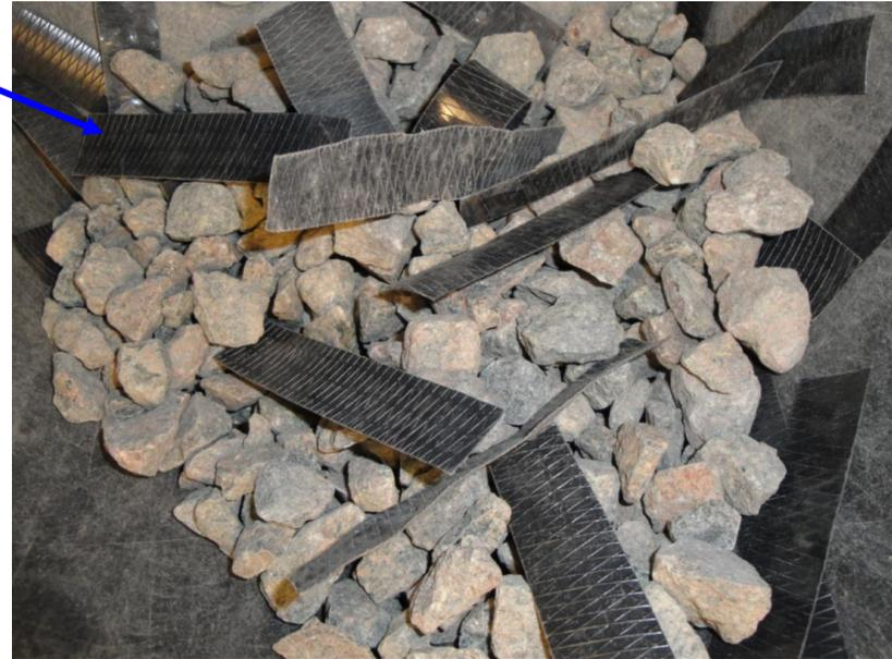
Fibre reinforced ballast
