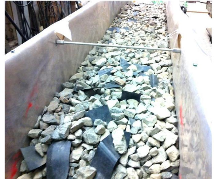
Fibre reinforced ballast
