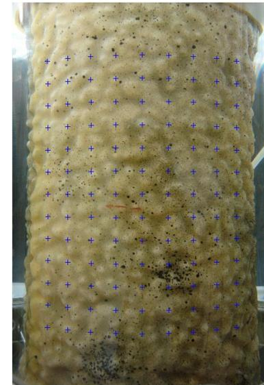
Measurement grids on triaxial specimen
