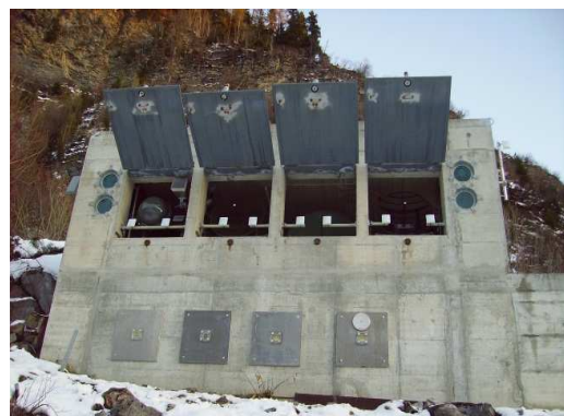
in the Vallée de la Sionne test path. Our radar receivers are the white rectangles in the windows
