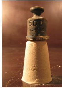
(b) Effect of suction on the mechanical resistance of sand.
