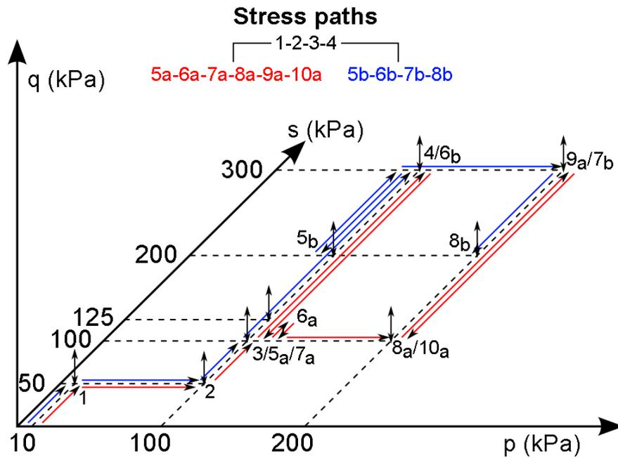
Figure 1: Applied stress paths; red - 70mm diameter, blue - 38mm diameter.
