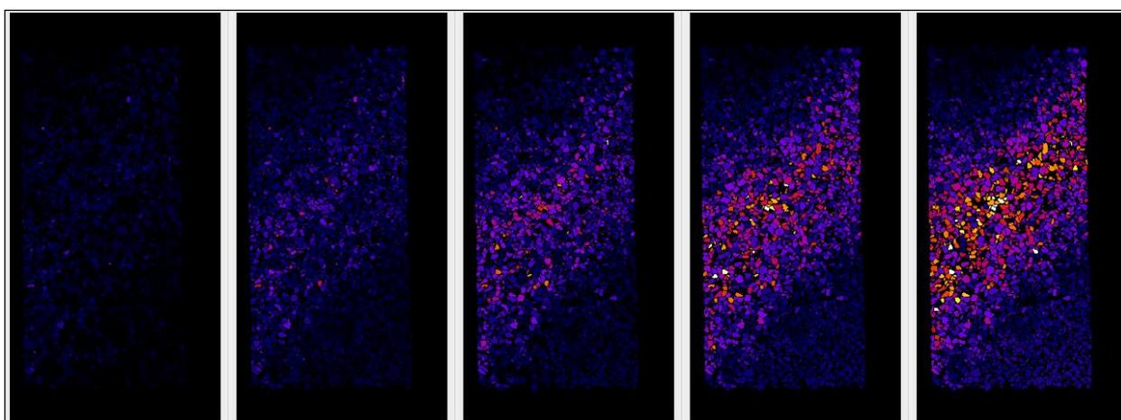
**Figure 5:** Vertical slices of Hostun sand specimen showing grain rotation measured over increments during the test. Grains are coloured by the value of their measured total rotation. Not all increments of the test are shown.
