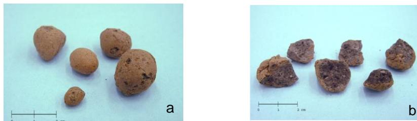
**Figure 1:** LECA pellets: (a) whole, (b) broken with intra porosity. (Casini et al, 2013)
