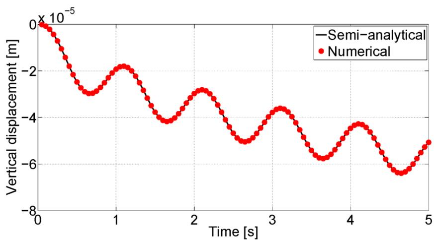
**Figure 3 :** Numerical versus semi-analytical vertical displacement at the top boundary for  $k=10^{-4}m/s$  .
