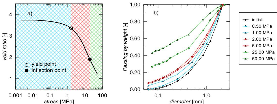
**Figure 2:** Experimental results: (a) compressibility curve, (b) evolution of grain size distribution.
