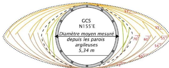
**Figure 4:** conceptual model of induced fractures and damaged zone at Andra URL for a tunnel excavated in a far-field stress state with weak anisotropy conditions. Modified after A.Noiret, Andra internal report, 2012.
