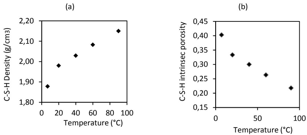
**Figure 1:** (a) Variation of C-S-H density and (b) C-S-H intrinsic porosity with temperature
