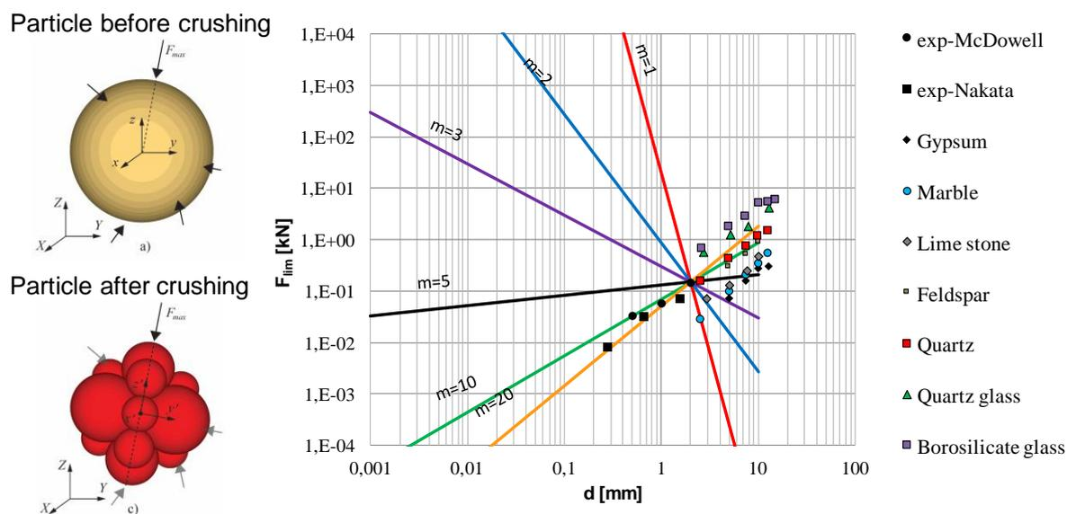
**Figure 1:** Particle limit contact force as a function of particle diameter, where  $F_{lim} = (lim_0)(d/Nd_0)^{-3/m}A$ . Also shown are single grain crushing experiments by Yashima et al. (1987), Nakata et al. (2001) and McDowell (2002) after Ciantia et al. (2015).
