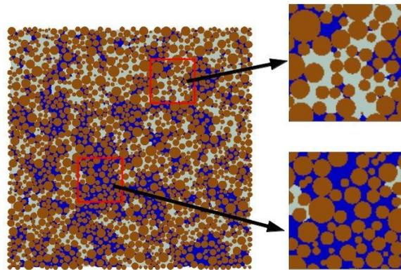
**Figure 1 :** A slice through a sample at 0.4 of saturation (the NW phase invades from the top and W phase recedes from the bottom), in which strong capillary fingering can be observed
