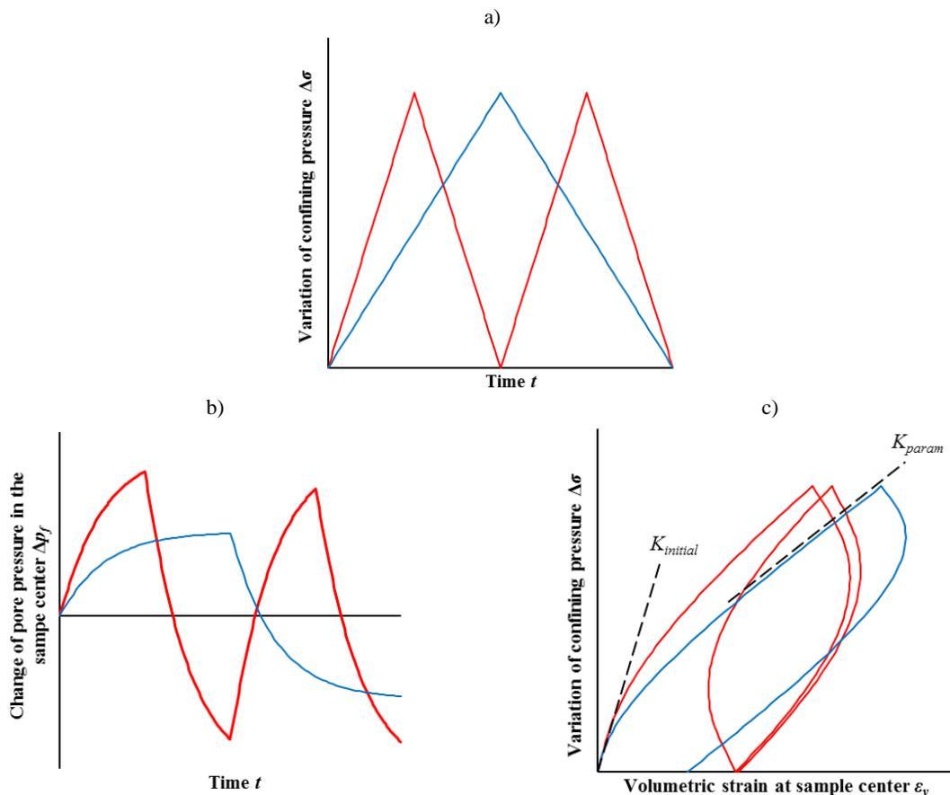
**Figure 1:** Exemplary simulation of drained test under two different loading rates (a), generated pore pressures (b) and resulting deformations (c).
