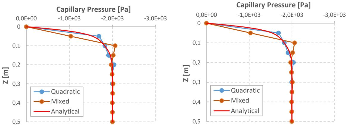
**Figure 1 :** Water pressure distribution along the height of the column for  $k = 10^{-5}$  m/s (left) and  $k = 10^{-13}$  m/s (right), at  $t = 0,15$  s.
