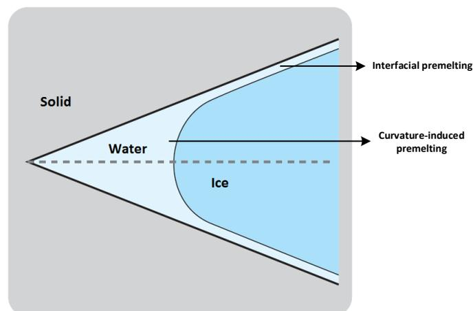
**Figure 2 :** Curvature induced premelting and interfacial premelting during intrusion of ice into a wedge-shaped wet preferential solid (Zhou, 2014)
