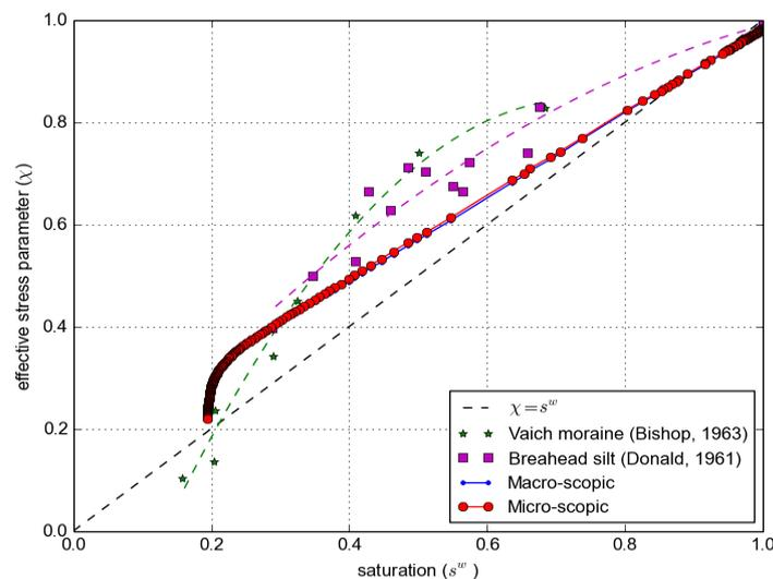
**Figure 2 :** Variation of effective stress parameter  $\chi$  with saturation for simulation results and experimental data. Simulation values are calculated from drainage test of a dense packing (40,000 spheres) under the oedometer test conditions.
