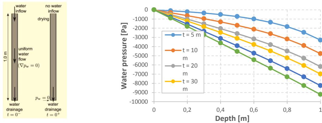
**Figure 2 :** I.C. and B.C of Liakopoulos experiment (left) and negative pore pressure evolution in time (right).
