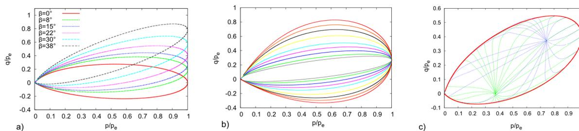
**Figure 2:** Results of the model: a) SBS of the newly developed model with various values of rotation, b) SBS rotated by  $\beta=22^\circ$  with various values of critical state friction angle (ranging from  $\varphi=14^\circ$  to  $\varphi=39^\circ$ ). c) Normalized stress paths starting from two arbitrary states leading to an asymptotic state, thus forming asymptotic state boundary surface.
