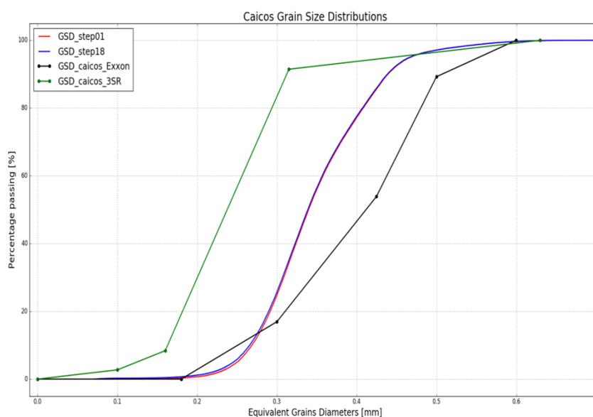
**Figure 4:** Grain Size Distribution comparison between sieve analysis (*GSD\_caicos\_Exxon*, *GSD\_caicos\_3SR*) and image analysis (*GSD\_step01*, *GSD\_step18*)
