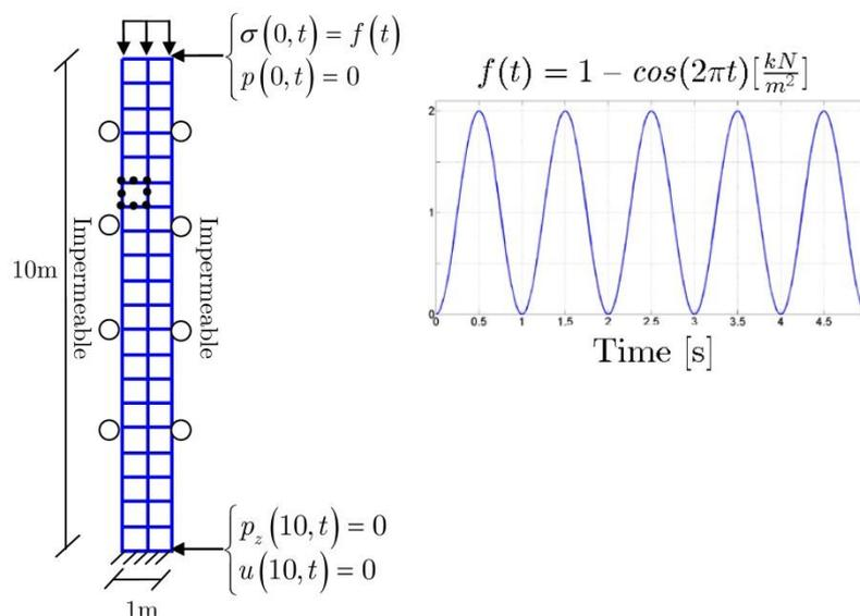
**Figure 1 :** Geometry, boundary conditions, mesh and loading path for the numerical simulation.
