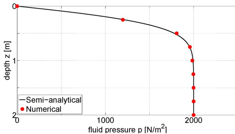
**Figure 2 :** Numerical versus semi-analytical pore pressure distribution with depth at  $t=0.5s$  for  $k=10^{-4}m/s$  .
