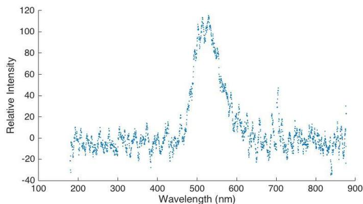
**Figure 1:** Mechano-luminescent emission spectrum of Europium-doped Molybdenum Aluminate (Sample 2)
