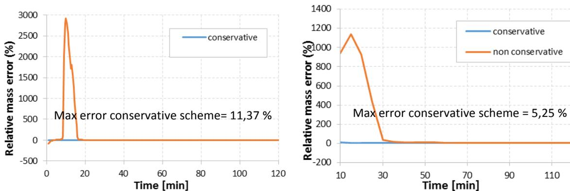
**Figure 3 :** Mass balance errors comparison using two different time stepping:  $\Delta t = 5$  min (left) and  $\Delta t = 30$  s (right).
