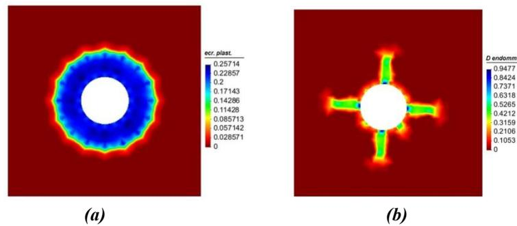
**Figure 1:** internal variable extension and values for the elastoplastic (a) and damage (b) softening models.
