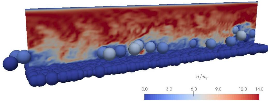
**Figure 1:** Instantaneous velocity field, particles and fluid.
