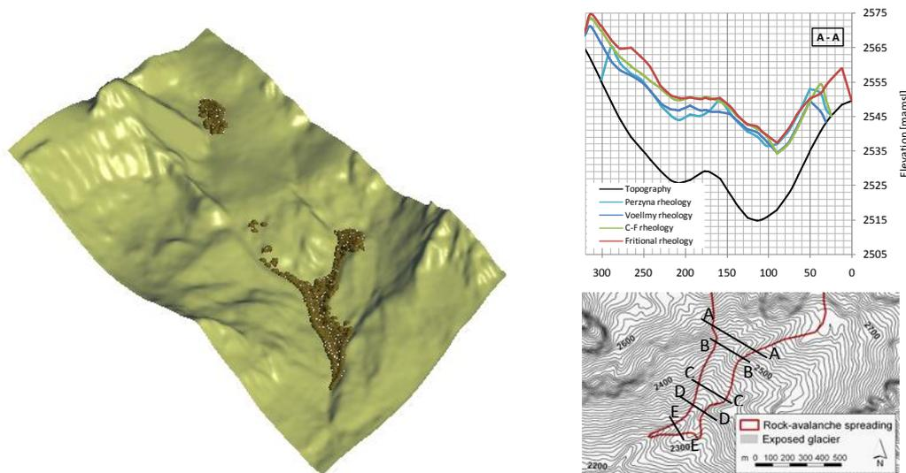
**Figure 1 :** Thurwieser avalanche: comparison of cross section for different rheological models and the propagation in 3D terrain for 90s for Perzyna rheological model.
