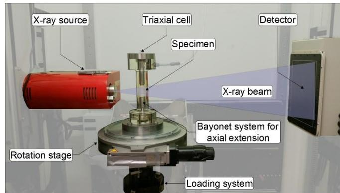
Figure 1: Setup of the triaxial equipment in the x-ray scanner.
