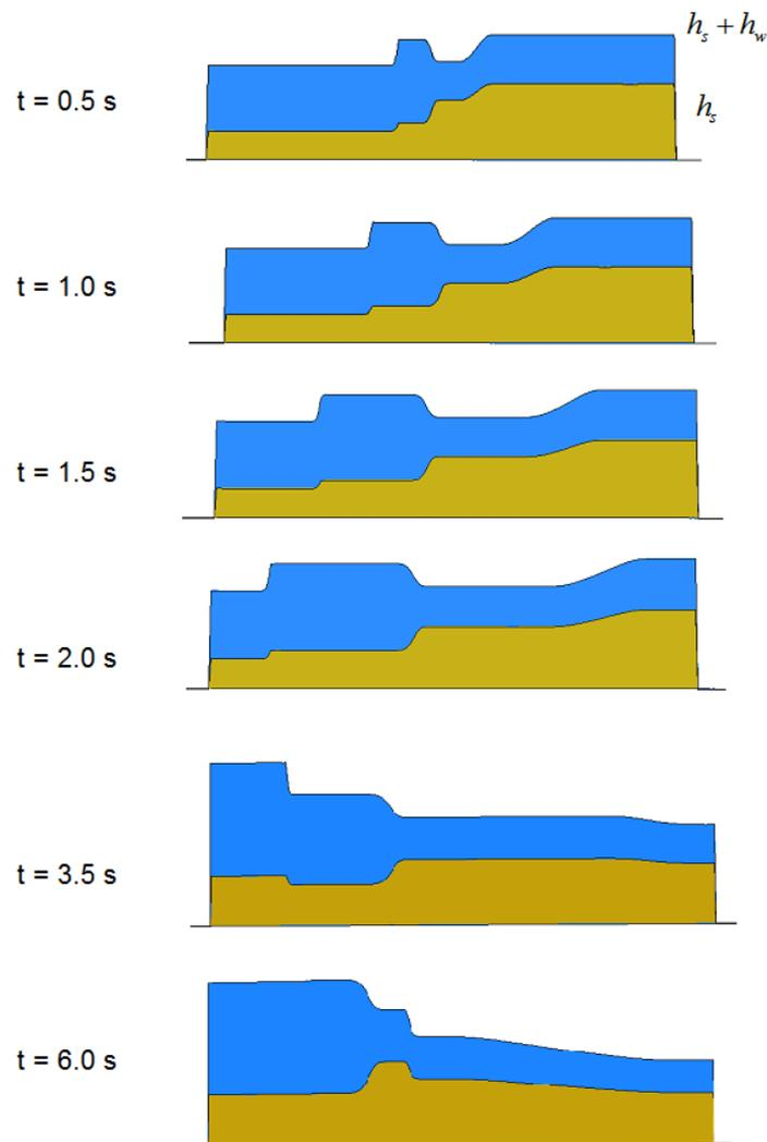
**Figure 2 : Profiles of  $h_s$  and  $h_s + h_w$  at times 0.5, 1.0, 1.5, 2.0, 3.5 and 6 s**
