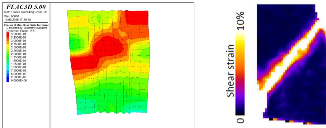
Figure 3: Comparison between numerical and experimental result.
