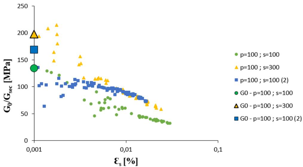
Figure 2: Effects of suction and its history on  $G_0$  and shear modulus reduction curve ; stress path = 3-4-5<sub>a</sub> (see Fig. 1).
