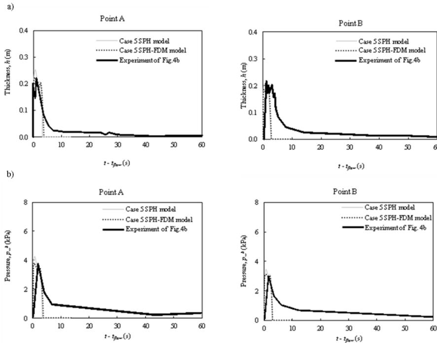
**Figure 1 :** Comparison of the flume test measurements and numerical simulations: a) evolution of flow depth ( $h$ ); and b) evolution of basal pore water pressure ( $p_w^b$ ) at the points A and B. The legend refers to the experiment of Fig. 4b and the numerical simulation of the Case 5 of Table 2 shown in the paper Cascini et al. (2016)
