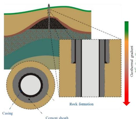
Figure 1 : Oil well schematic representation.
