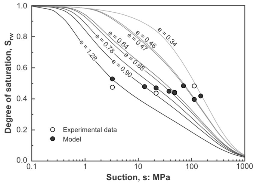
**Figure 1:** Comparison between experimental data (Gatabin et al. 2016) and model predictions. Wetting path under unconfined conditions.
