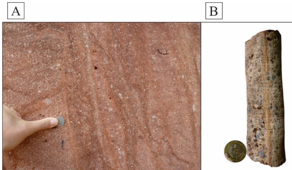
Figure 1: a. Material exposed to the outcrop; the thumb is places next to a deformation band; b. plug coming form (a).
