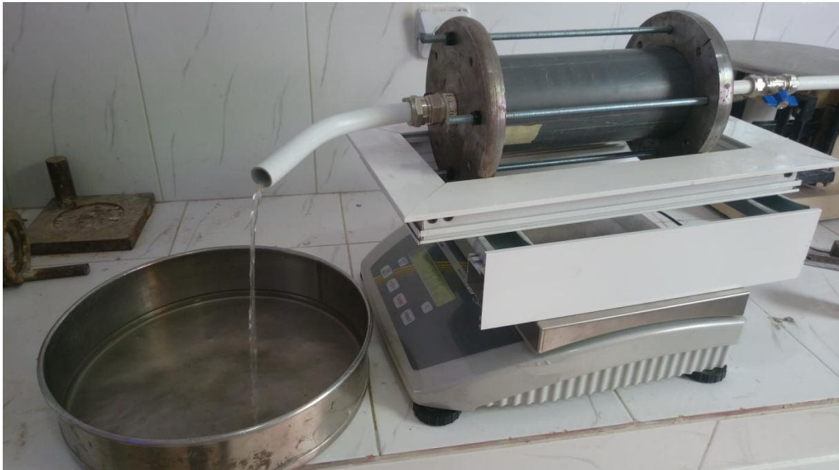
Figure 1: the erosion cell
