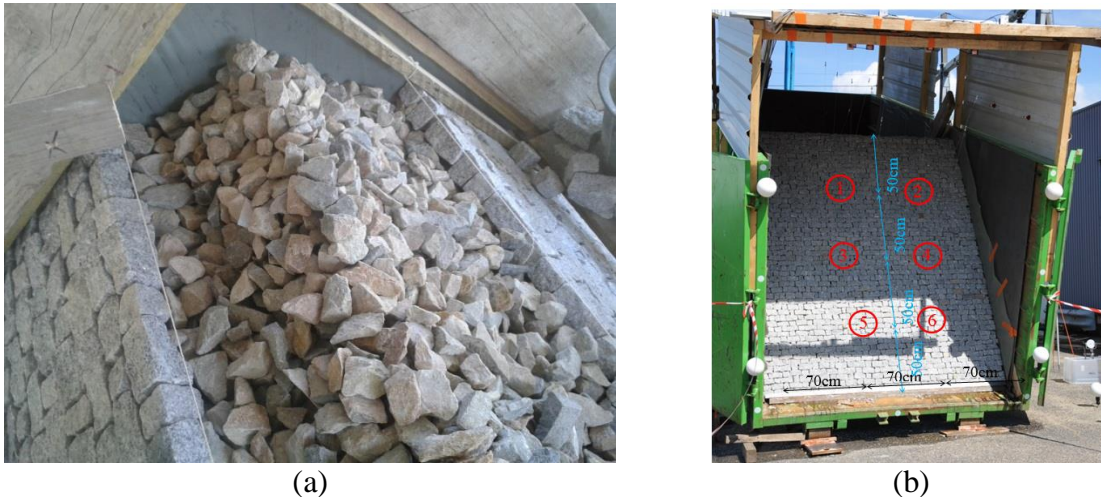
Figure 2: Scaled-down rockfill dam: (a) construction; (b) mock-up installed in a truck box which is progressively inclined
