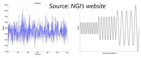
Converting pseudo-random loading into equivalent harmonic load packets.
