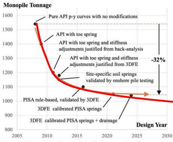
Figure 12. Achieved material efficiency gains due to geotechnical design evolution.
