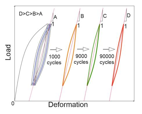
Stiffness degradation and loss of strength
