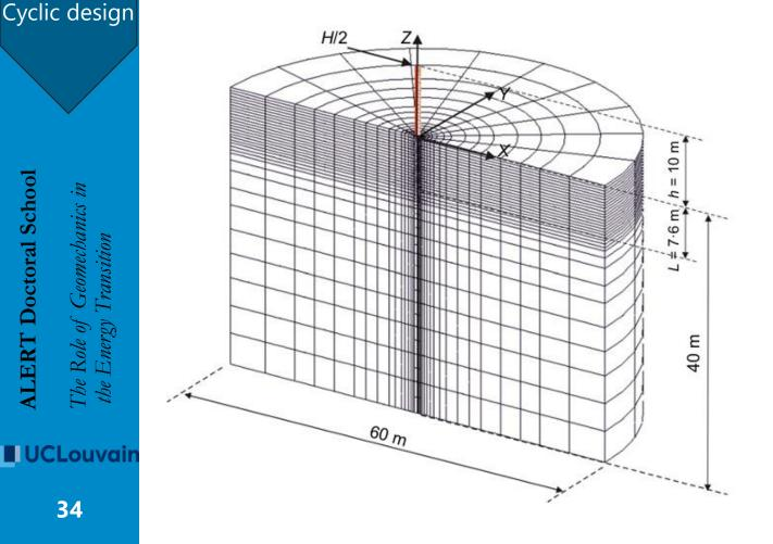
To model the macro-scale phenomena, one needs <u>advanced constitutive models capable</u> of capturing cyclic behaviour of the soil at the meso-scale for the different stress paths and amplitudes that will be sustained by the OWT surrounding soil.
