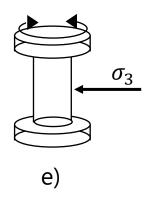
Resonant column Small-strain Behaviour.
