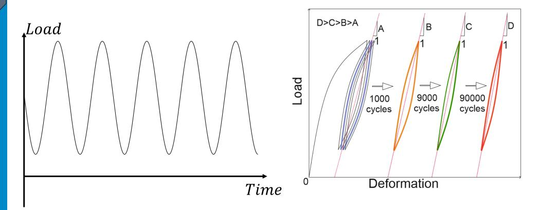
Ratcheting: accumulation of strain/deformation/displacement.
