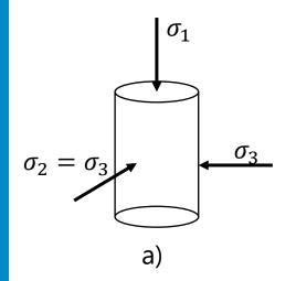
Triaxial Axisymmetric Stress state
