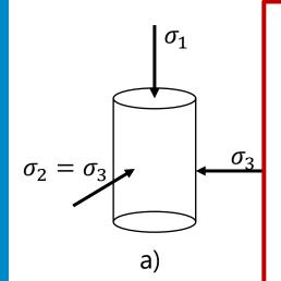
Triaxial Axisymmetric Stress state
