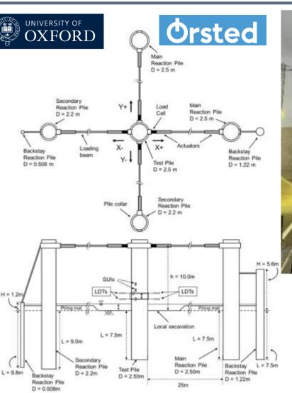
Figure 4. Schematic for large diameter multi-directional cyclic test (P09). Source: *Byrne et al. (2025)*
