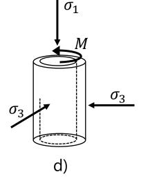
Hollow cylinder Torsional test Control three principal stresses + stress rotation.
