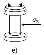
Resonant column Small-strain Behaviour.
