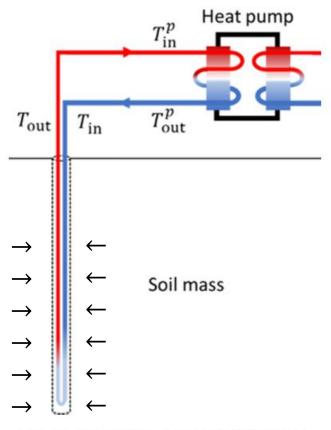
Fig. 12. Heat pump - heat exchanger set-up.
